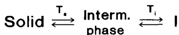
Figure 8 Scheme of the phase behaviour in PTA12HQ12 powders. Upon heating the solid room-temperature phase to above the side-chain melting temperature T_s , an intermediate phase is formed, which transforms to the isotropic melt at the clearing temperature T_i
